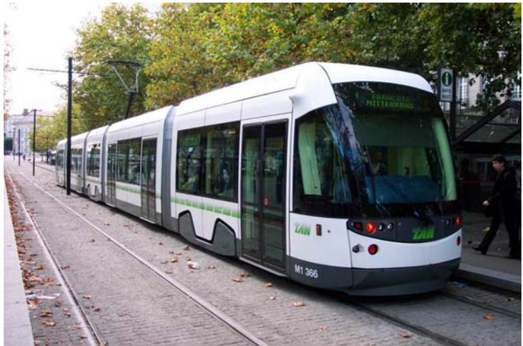
In order to achieve the lowest possible floor level, electrical equipment was switched to the roof area. Narrower seats and the removal of interior steps have created more circulation and boarding room in order to reduce station dwell time.
