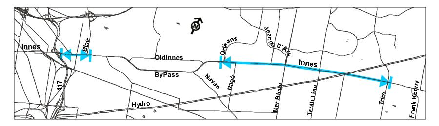
West Section Proposed widening from 4 to 6 lanes (1.2 km) East Section Proposed widening from 2 to 4 lanes (6.5 km)
