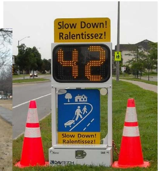
Two examples of how a mobile speed trailer is used to help with education and enforcement by indicating drivers' current speed in relation to the posted speed limit. (City of Ottawa)
