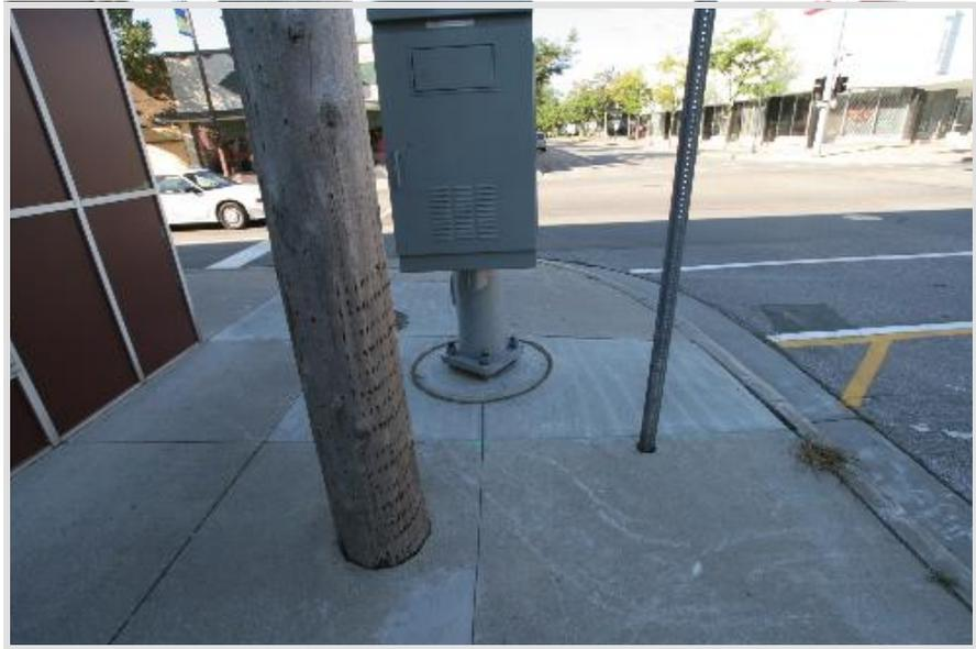
Obstacles such as hydro poles, utility cabinets, and street furniture can seriously impede sightlines between drivers and pedestrians at intersections. They can also impact the refuge area available when waiting for signals, especially for pedestrians in wheelchairs ([www.pedbikeimages.org/](http://www.pedbikeimages.org/) Dan Burden).
