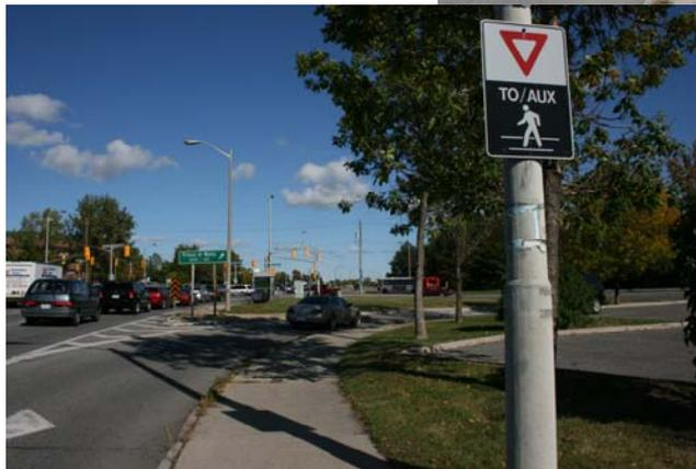
In the example above a sign blocks the driver's ability to see pedestrians crossing at the crosswalk. The example at left illustrates the sightline limitations to the crosswalk due to vegetation. Both of these obstacles are located at the same crosswalk and are relatively inexpensive to remedy. (McCormick Rankin Corporation)
