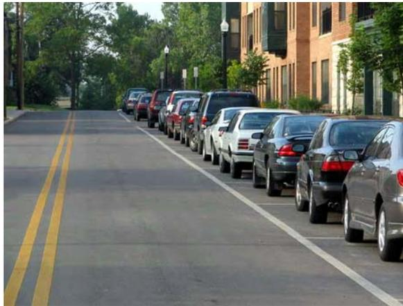
An example of on-street parking. It provides a buffer between traffic and pedestrians and narrows the roadway—helping to reduce vehicle speeds. However, on-street parking can limit the visibility of pedestrians. ([www.pedbikeimages.org/](http://www.pedbikeimages.org/) Dan Burden)
