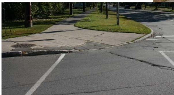
An example of deteriorated pavement and concrete surfaces is shown at left. The result of poor maintenance is shown above where standing water is located in the crosswalk. These types of conditions can be a hazard to pedestrians and increases agency liability. ([www.pedbikeimages.org](http://www.pedbikeimages.org/) / Dan Burden / McCormick Rankin Corporation)
