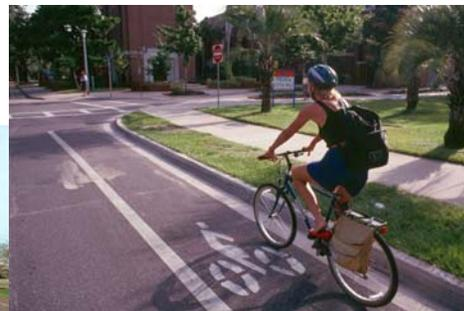
The photo above shows how a bicycle lane can provide a buffer between vehicles and pedestrians. The photo at left illustrates how bicycle lanes help narrow the travel lanes and may help to reduce vehicle speeds.
