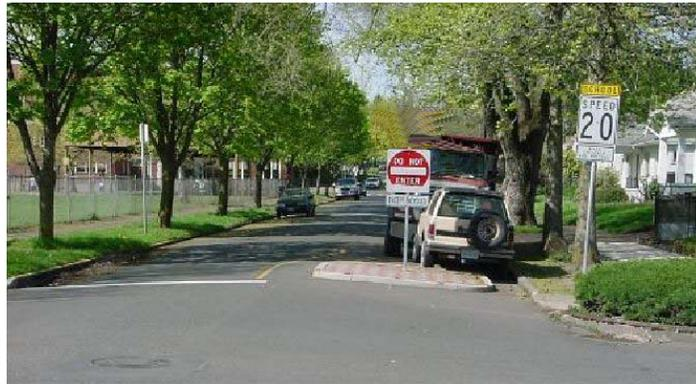
This is an example of a partial intersection closure that prevents vehicles from entering the street. As a note, the signage illustrated here is not consistent with the practices of the City of Ottawa for this type of treatment. ([www.pedbikeimages.org](http://www.pedbikeimages.org/) / Dan Burden).
