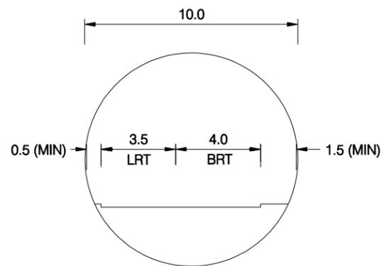
10.0m BRT / LRT TUNNEL
