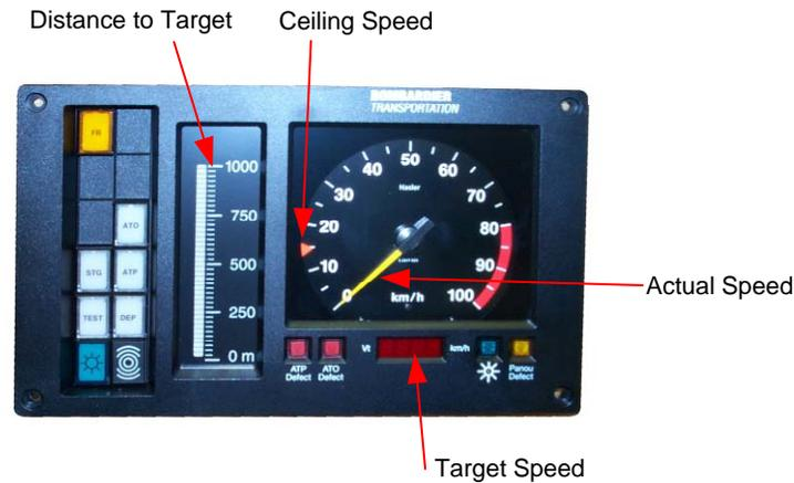
Figure 9 - Typical Cab Display
