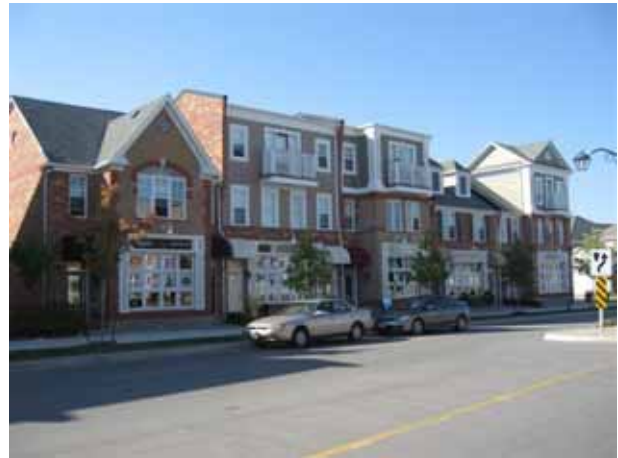
Live-work townhouses have their ground floor designed to be either a store or professional office, or part of a home. Their location right on the sidewalk creates the possibility for these buildings to evolve over time as either people's homes or part of a mixed-use street. Courtesy: Mattamy Homes
