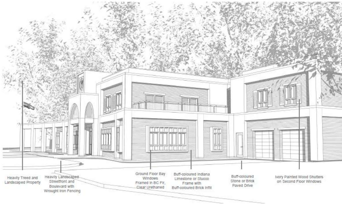
Figure 4: Presentation drawing of the main elevation, the north elevation and the garage entrance, with annotations concerning materials. Drawings provided by Julian Jacobs Architects Inc., 17 Feb 2012.
