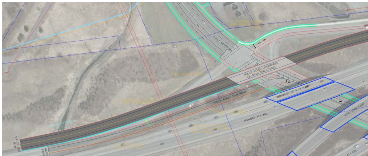
Figure 2-5: Alternative B2 – Over Holly Acres with Relocated Highway Ramp
