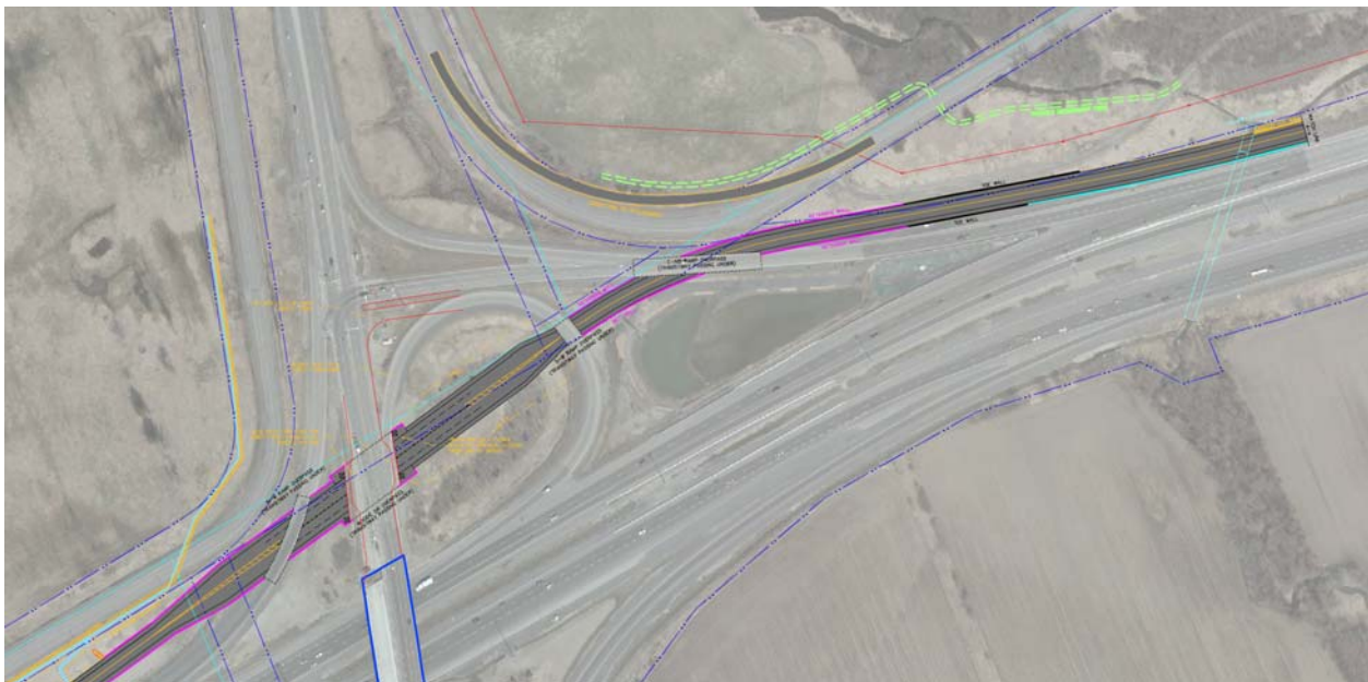
Figure 2-10: Alternative B1 - Alignment Through the Moodie Drive Interchange and Under Moodie Drive with a Station on Moodie Drive
