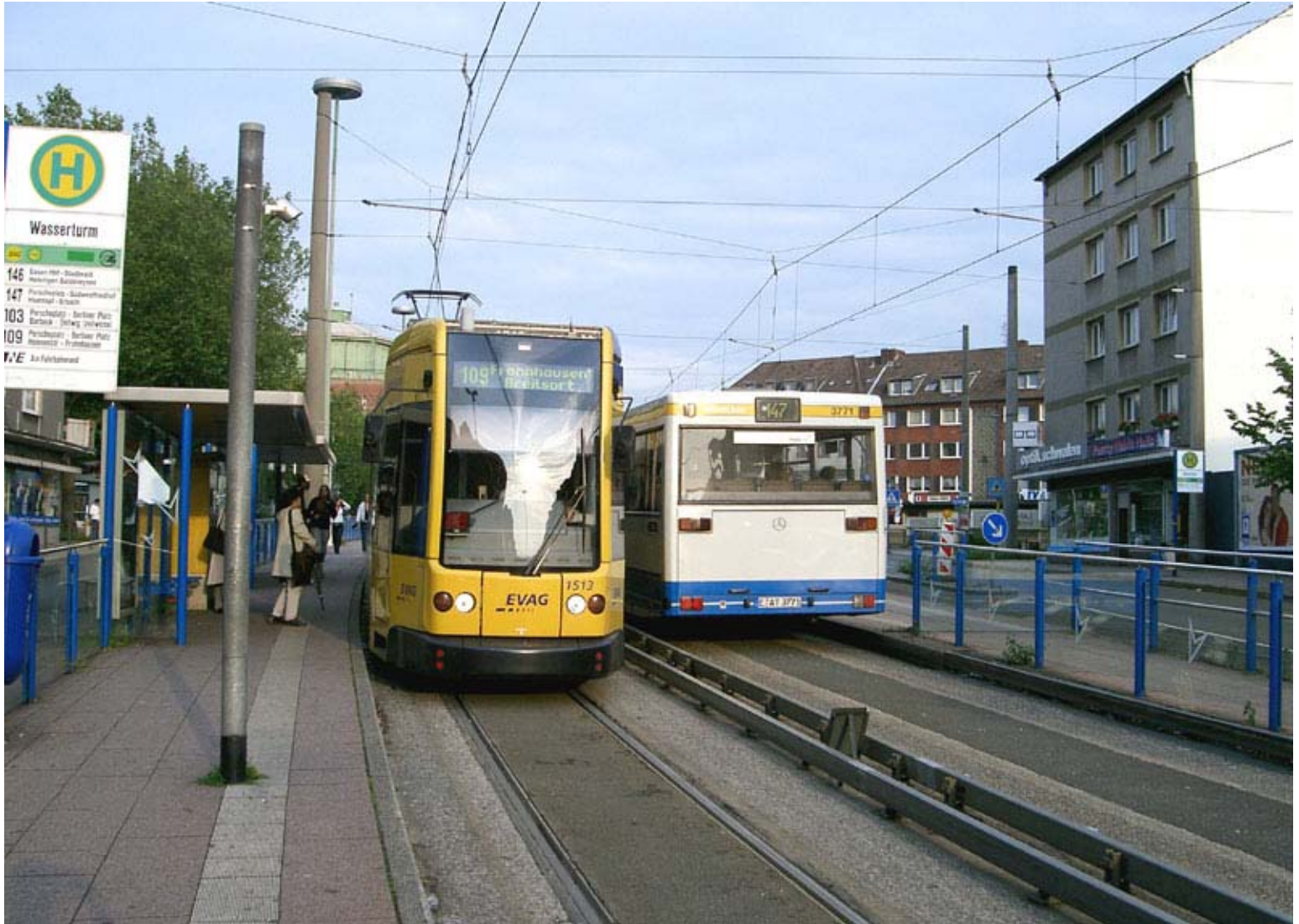
Essen Germany: the operation of guided buses and LRT on the same alignment using common signaling. (The use of shared RoW has been implemented in a number of German cities due to street space limitations.) This is similar to the proposed BRT/LRT joint operation on the Transitway.
