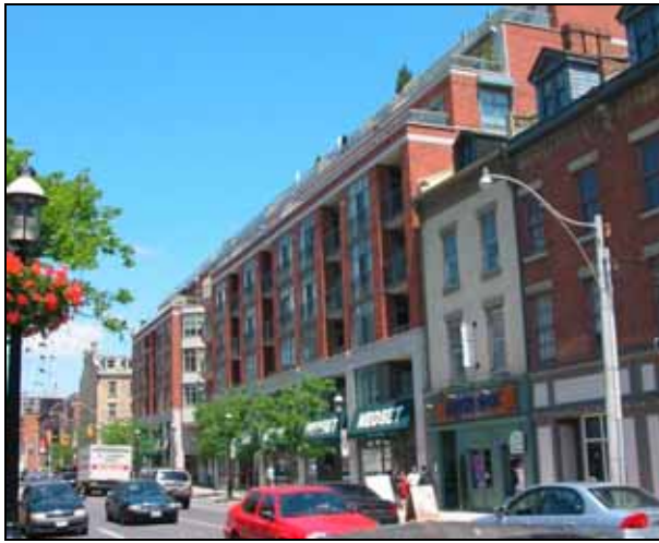
Figure 11: Buildings set back above 3-4 storeys preserve a human scale and allow more light to reach the sidewalk.
