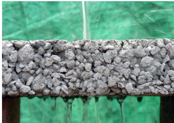
Figure 5b: Cross-Sectional View of Porous Asphalt 12
