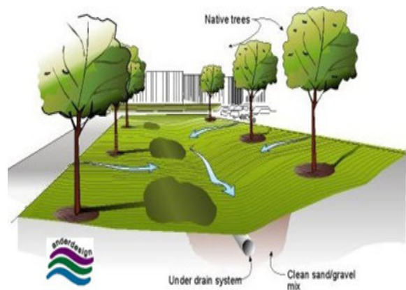
Figure 6b: Digital Rendition of a Grass Swale with Sub-Drain 14
