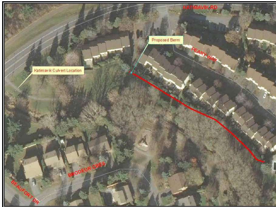
Figure 6 – Proposed Berm Behind Homes on Peary Way
