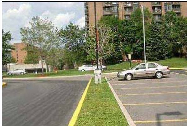
Figure 15: A grassed curb separates the stacking lane from parking areas in this drive-through site.
